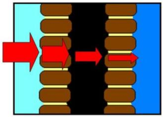
Most outside walls have an empty space between the 2 layers of bricks called a *cavity*. This reduces heat loss by *conduction* through the bricks.
