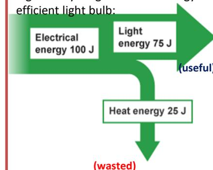
**Efficiency** is a measure of how much of the energy supplied to a device is transferred into useful energy.
