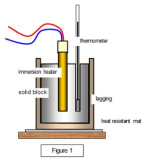
1. Use a top-pan balance to measure the mass of the block.
