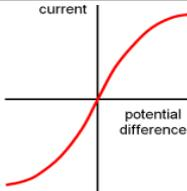
The current through a **diode** flows in one direction. It has a very high resistance in the opposite direction.
