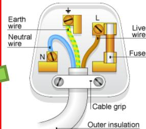
The circuits in your house are earthed outside. Appliances with metal cases need to be earthed inside the case. This is just in case a live wire comes loose- the current will then pass through the earth wire and not you when you touch it.
