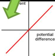
The resistance of a **bulb** increases as the temperature of the filament increases
