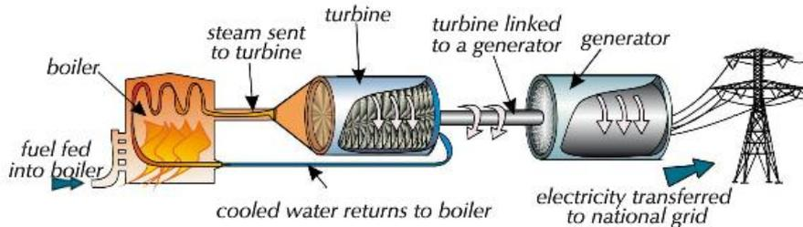
Figure 3: Electricity generation in a fossil fuel power station.
